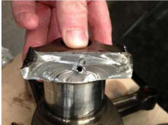
So, which was it? It's almost impossible to say for sure, but either way, the shop doing the overhaul had an obligation to perform a thorough inspection of the crank. The reason that a crank is inspected during an overhaul is specifically to PREVENT a fatigue failure by identifying any flaw that could lead to this catastrophic failure mechanism. The inspection is your ONLY opportunity to avoid such a failure.
